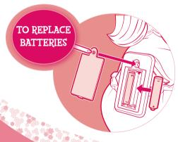
Use a Philips/cross head screwdriver (not included) to loosen screw in battery compartment cover (screw remains attached to cover). Remove cover. Remove and discard old batteries. Replace with fresh 2 x 1.5V "AAA" or RO3 size batteries. Alkaline batteries recommended. Replace cover and tighten screw.
